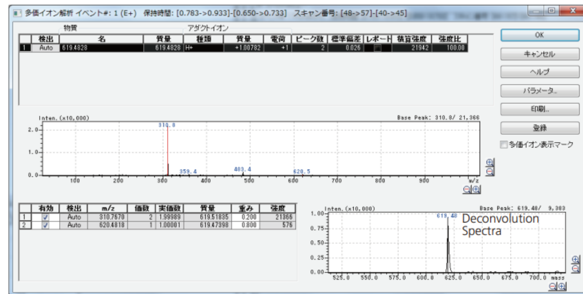
Fig. 3 不純物の多価イオン解析結果 Result of Deconvolution with Respect to Major Impurity
